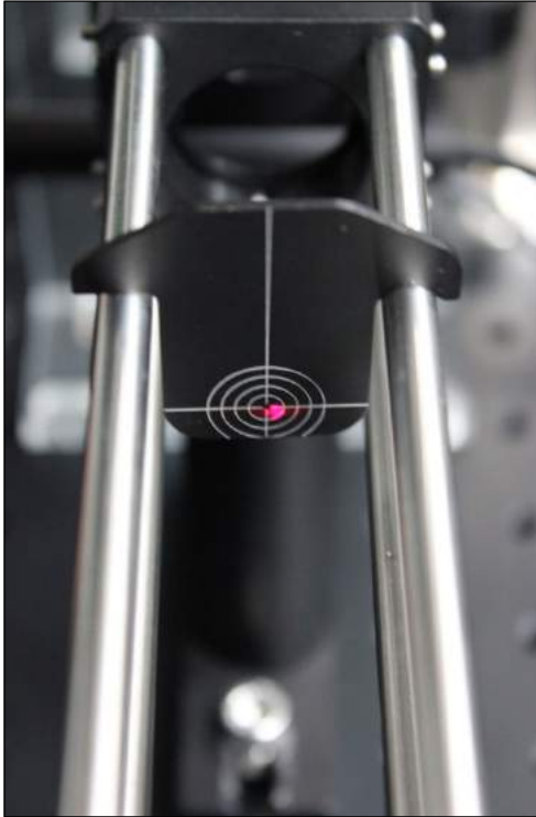
Figure 49 Laser Spot on the CPA1 Cage Alignment Tool
