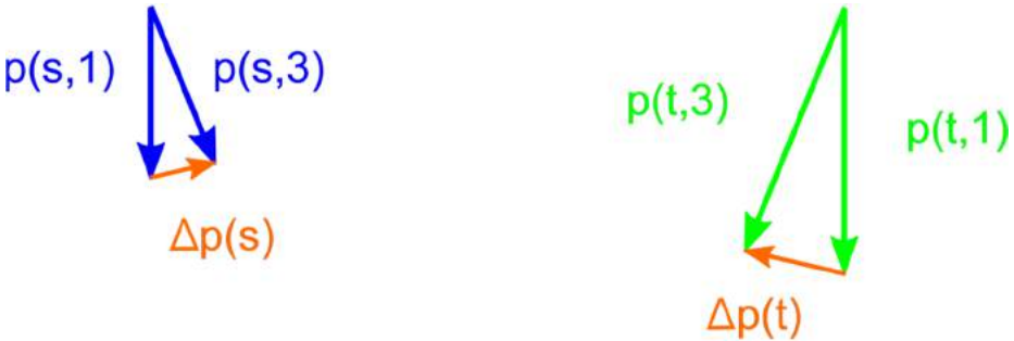
Figure 66 Unfocused Off-Axis Laser Beam Momentum Changes
