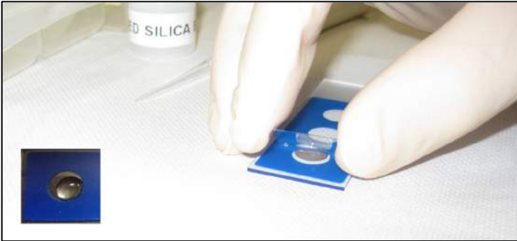
Figure 53 Droplet of Bead Solution on Glass Slide
